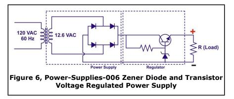
In the circuit shown in Figure "Power-Supplies-006", the current capacity of the regulator is greatly increased by the use of the transistor. The base of the transistor is kept at a constant voltage by the zener diode. The base emitter junction drops about 0.5 to 0.7 volts. Therefore the voltage across the load will be about 0.5 to 0.7 volts higher than the zener voltage.
