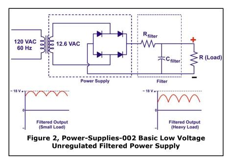
d. The value of R<sub>filter</sub> is typically less than one tenth of the load resistance.
