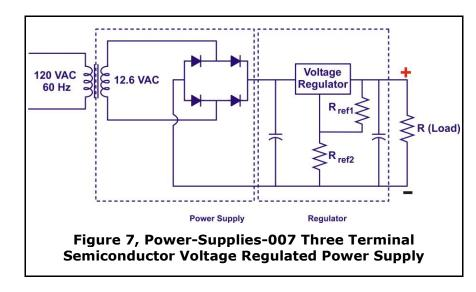
4. Integrated Circuit Voltage Regulator Circuits
