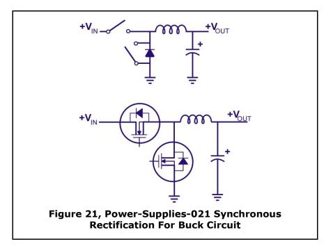
ss. Skip Mode Improves Light Load Efficiency: A feature offered in many modern switching controllers is skip mode. Skip mode allows the regulator to skip cycles when they are not needed, which greatly improves efficiency at light loads. For the standard buck circuit (Figure "Power-Supplies-012") with a rectifying diode, not initiating a new cycle simply allows the inductor current or inductor energy to discharge to zero. At this point the diode blocks any reverse-inductor current flow and
