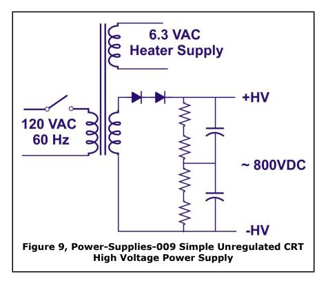
a. The circuit in Figure "Power-Supplies-009" supplies high (~800VDC) to a Cathode-Ray Tube (CRT). The CRT current demands very small and does not change (for all practical purposes). Therefore the ripple is negligible and the voltage level is very steady. Since the voltage is very steady, no
